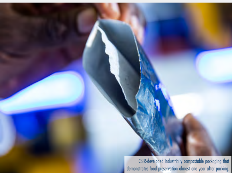
The packaging blocks oxygen, thereby preventing spoilage and extending shelf-life.
