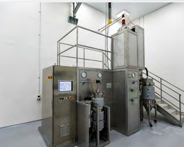
The supercritical CO 2 microencapsulation facility for enhancing the therapeutic benefit of nutraceuticals and offering compound micronisation with tailored particle characteristics.
